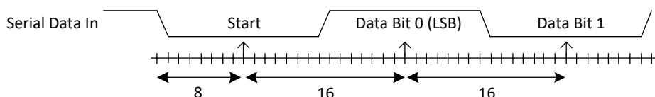
Figure 45: Receiver Serial Data Sampling Points
