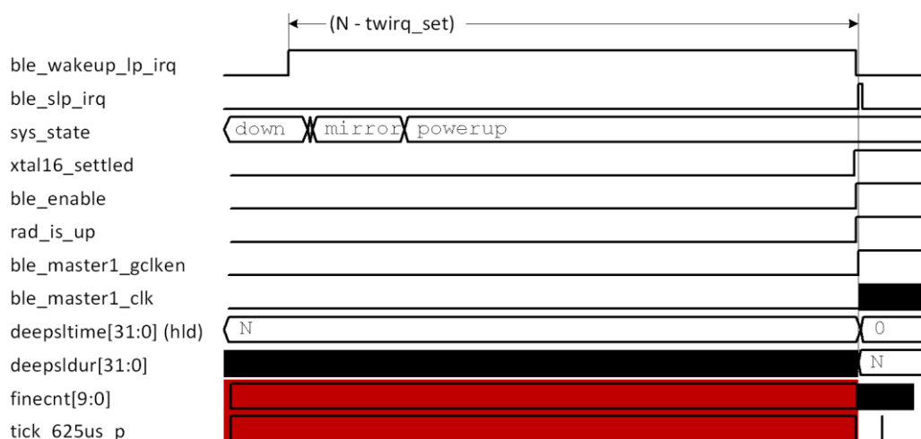
Figure 81: Exit BLE Deep Sleep Mode at Predetermined Time (Zoom Out)
