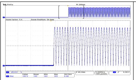
Test Condition: 135Vac with LED load
