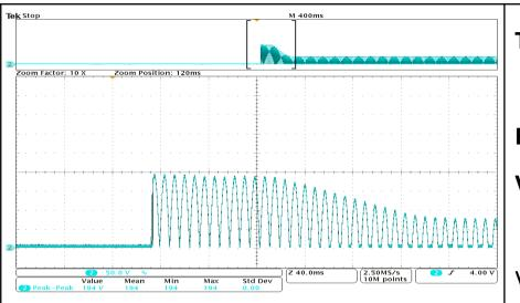
Test Condition: 135Vac with LED load
